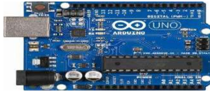
Figure 1: Arduino/Genuino Uno board based on the ATmega328P
