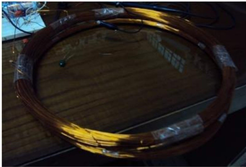
Fig. 4: Transmitter and receiver coil
