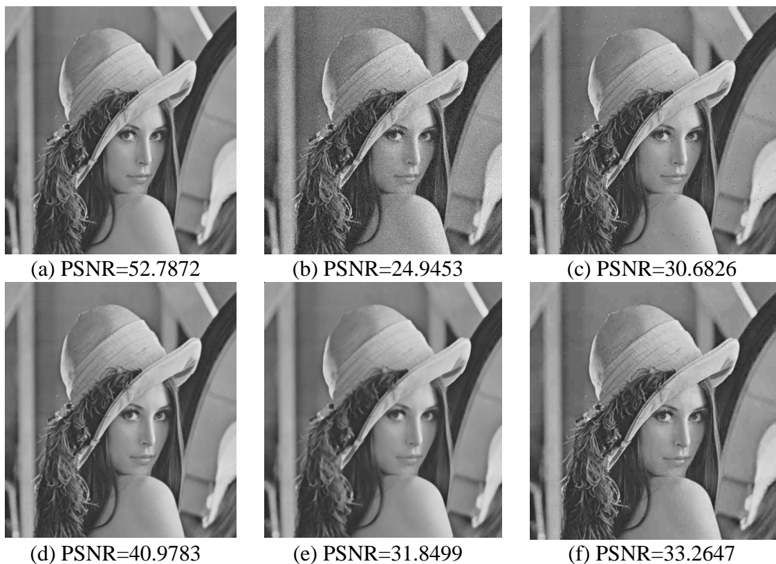
Fig.5: (a) watermarked Lena image (without attack), (b) attacked by Gaussian noise (mean=0, variance=0.006), (c) attacked by Salt & Pepper noise (mean=0,
