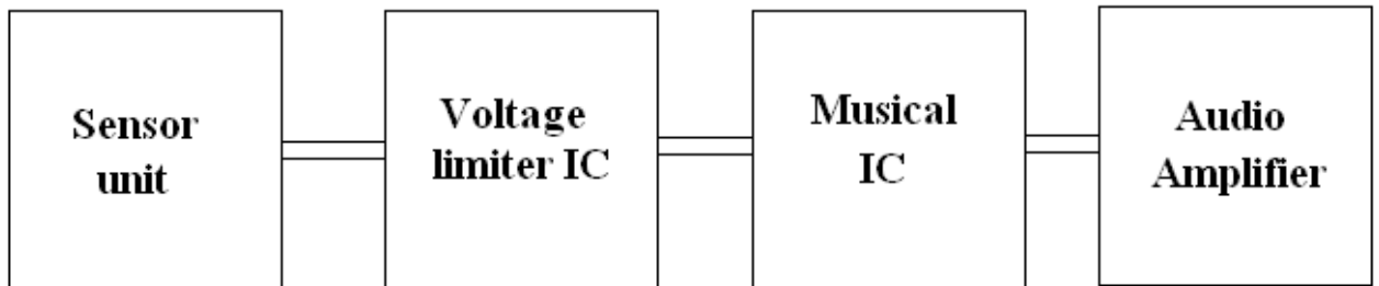
Fig. 4: Block diagram of detector unit
